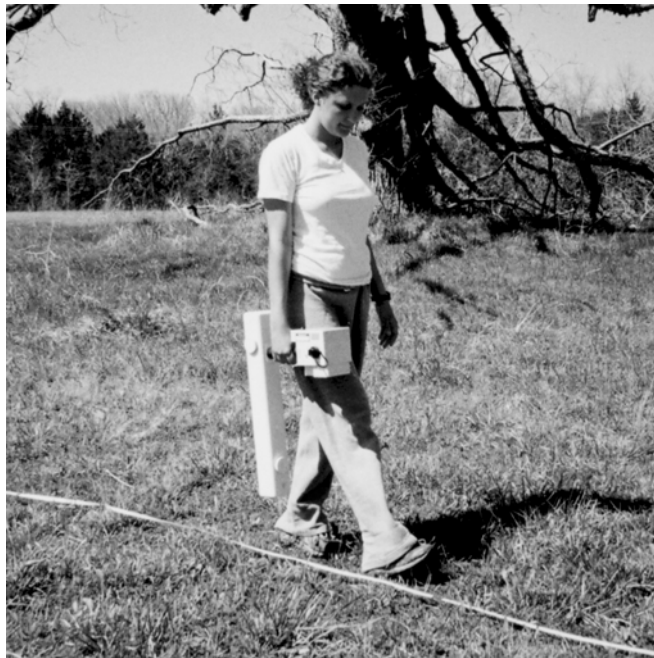
Figure 1. A magnetic gradiometer being used by a student from Mississippi State University at the Lyon's Bluff archaeological site in Oktibbeha county, Mississippi
